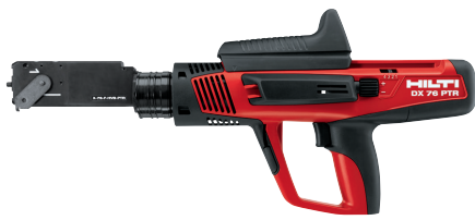
Figure 11: Hilti DX 76 PTR tool, equipped for X-HVB installation
