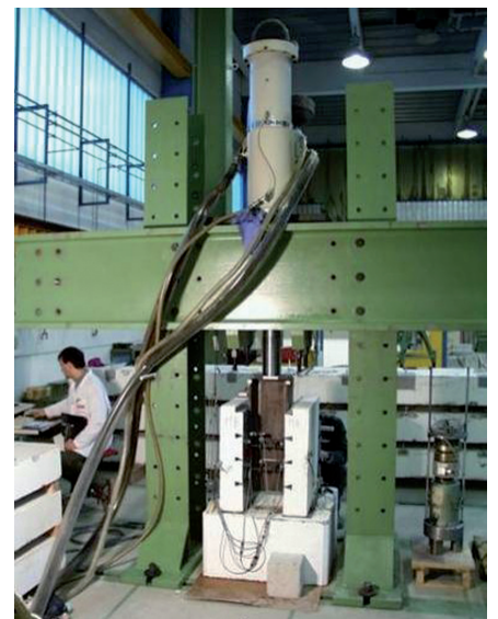
Figure 29: Push-out test with X-HVB
